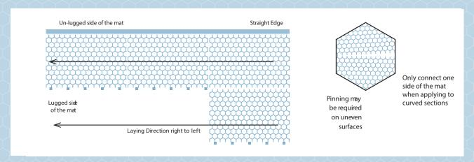
When applied to curved sections, only connect one side of the mat (only if entire connection is not possible)
